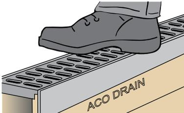
3. **To remove first grate**, insert grate removal tool (Part No. 01318) through slot at the end of grate and pull up sharply. Subsequent grates can be removed by hand (use gloves) – grip end of grate and lift.
