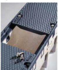
The CS system is supplied with heavy duty ductile iron lids in 500mm lengths. Each lid is secured with four high tensile steel bolts, incorporating friction grip washers to deter the bolts from working loose under vibration.
