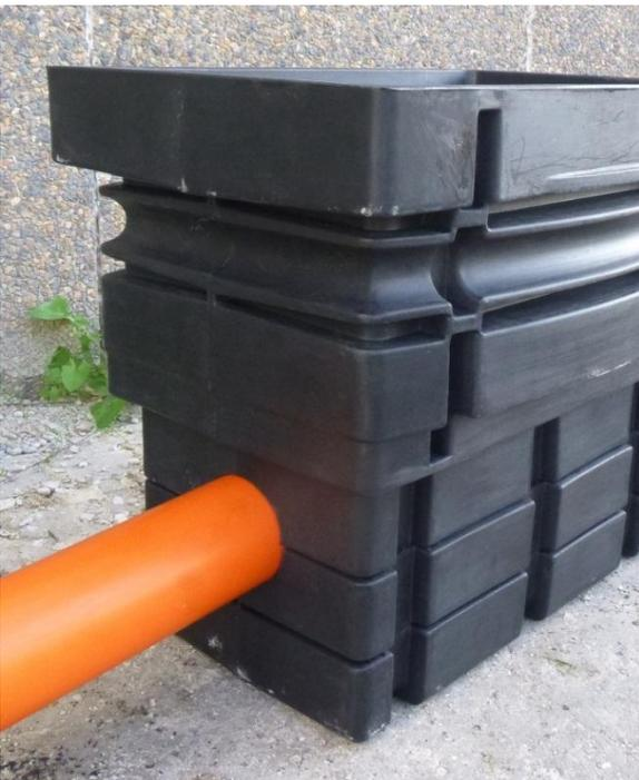
5. Using self-tap screws fix the two sections back together from inside the pit. Use a minimum of 8 screws spaced evenly around the retroribs.
