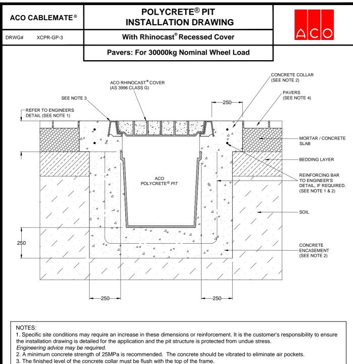
4. The paver course adjacent to the concrete collar must be flush with the collar and must be fully bonded to the mortar/concrete slab. 5. Refer to ACO's latest installation instructions for complete details.
