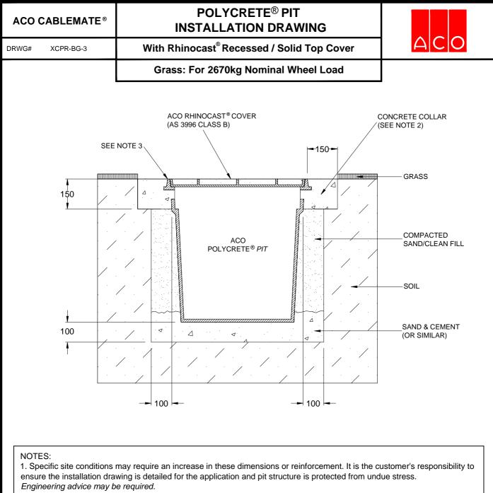
2. A minimum concrete strength of 25MPa is recommended for the collar. The concrete should be vibrated to eliminate air pockets.
